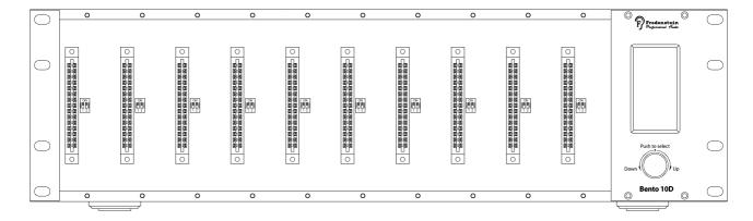
If certain non-Fredenstein modules are used, which bridge several pins on the connector and connected the contacts on the top and button side, the double switches, located directly besides the slot connectors, can both be turned off (lower position) to avoid interference between the module and the digital interconnect. For Fredenstein modules, both need to be in the ON (upper) position.
