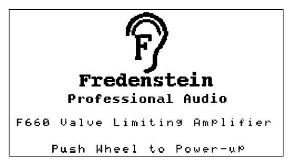
At this point the unit is in stand-by mode and the audio circuitry and the tubes are still powered-off, the unit is in bypass mode, but the output meter is connected to the main output. This allows the user to measure the level even in bypass mode.
