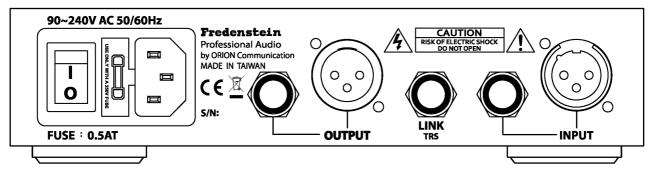
Please connect your audio inputs and outputs first to the XLR or TRS connectors located on the back panel. If you own two V.A.S. Comps, please insert a standard TRS cable into link connectors on both units. Connect the mains cable to the V.A.S. Comp and then to a grounded mains outlet. The power ON/OFF switch is located on the back panel near the power cable connector (IEC). After the unit is powered on, the PWR indicator on the front panel will be illuminated.
