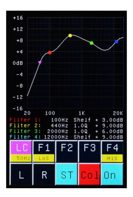
In the upper part of the screen, the frequency response of the F610 is plotted. Please note: the vertical axis automatically re-scales to up to +/- 64 dB. Touching the screen in the graph area switches to the spectrum analyzer mode (see details in the analyzer section of this manual, page 7). The horizontal frequency axis is displayed on a logarithmic scale.
