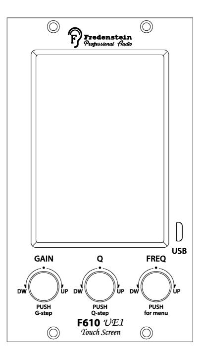
The user interface of the F610 UE-1 consists of a 3.5 inch TFT LCD touch screen with a resolution of 320 by 480 pixels. The touch screen is capacitive for superior precision and responsiveness. In addition, three rotary encoder for gain, Q-factor, and filter frequencies provide a traditional user interface for the most important parameters.
