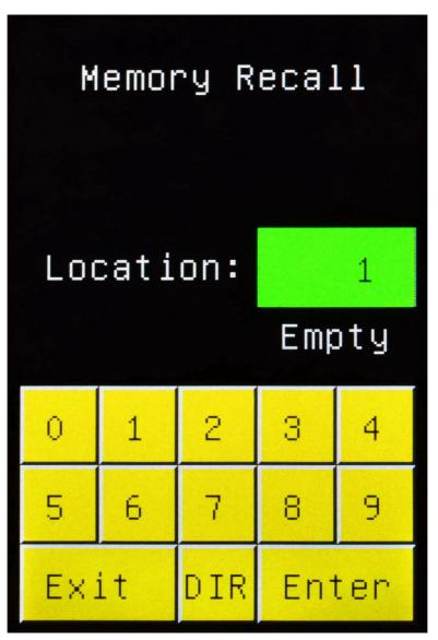
The user can input the desired memory location either by keyboard or by selecting the DIR directory listing. When using the keyboard, please always enter two digits, for number 1 please enter 01, etc. The status of the selected memory location is indicated by either an "Empty" or "Used" reference.
