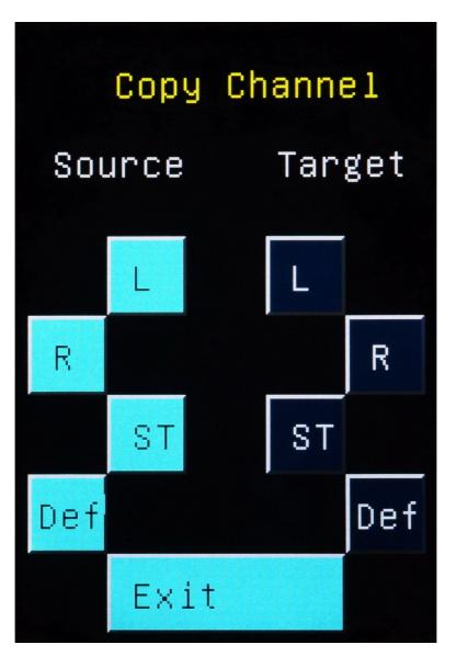
This menu allows for copying of channel settings. First select a source channel on the left side and then a destination channel on the right. The Def channel is a user defined channel setting, i.e. your favorite starting point for equalization. It must be stored first, the factory default sets all filters to 0 dB gain.
