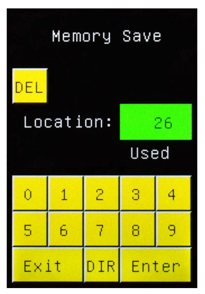
The user can input the desired memory location either by keyboard or by selecting the DIR directory listing. When using the keyboard, please always enter two digits, for number 1 please enter 01, etc. The status of the selected memory location is indicated by either an "Empty" or "Used" reference.
